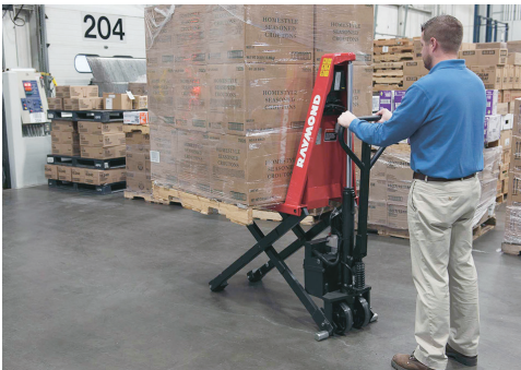
The truck's solid steel scissor legs provide maximum strength and rigidity under load.
